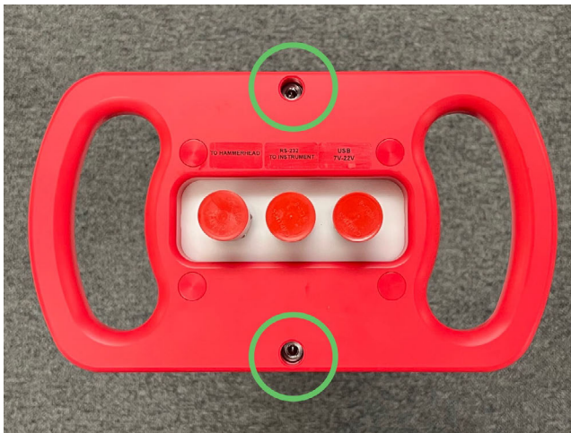
Fig. 11. Retaining bolts, tightened to 1.7N-m
