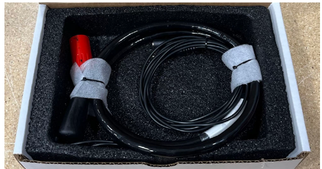
Fig. 4. MCBH-6FS inductive test loop cable
