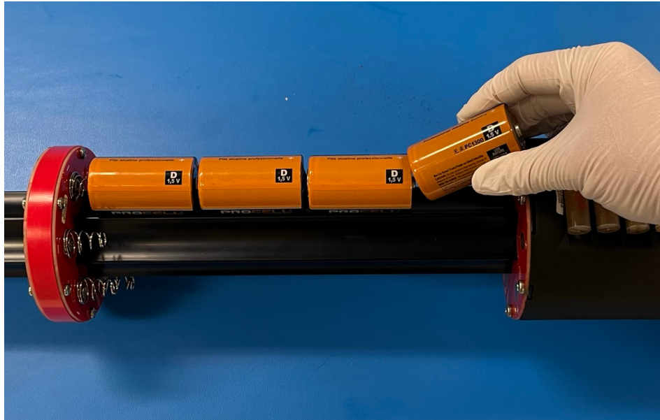
Fig. 20. Batteries' positive terminals face the battery end-cap
