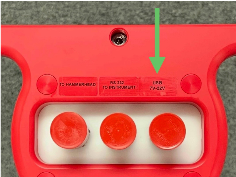
Fig. 15. MCBH-6-MP USB port position
