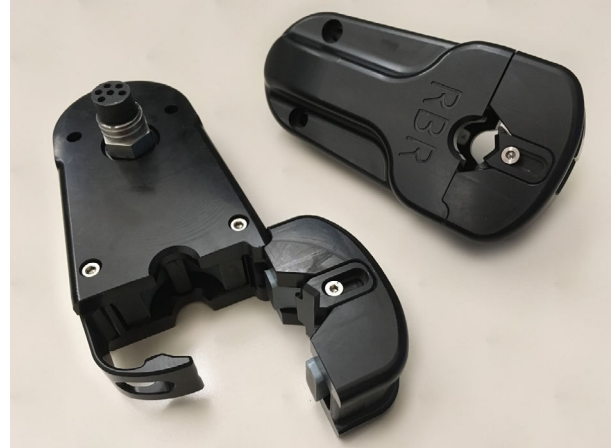
Fig. 27. Open and closed ferrite holders
