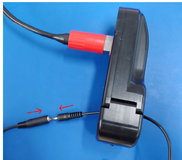
Fig. 26. "TO HAMMERHEAD" port
