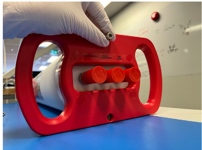
Fig. 12. Remove retaining screws with the RBRcervata lying on one side
