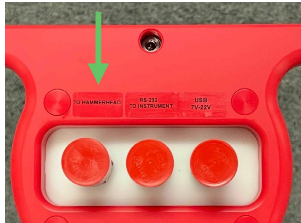
Fig. 26. "TO HAMMERHEAD" port
