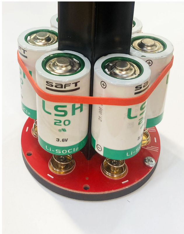
Fig. 21. Lithium batteries retained in carousel
