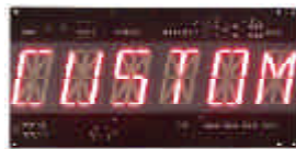
8100-0058 2.3-Inch, 16-Segment, Six Character Display, Red Super-Bright LED. Green and Yellow are optional
