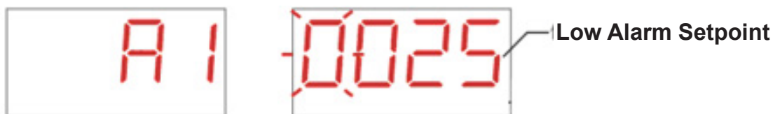
Low-Limit Alarm Setpoint Screen
