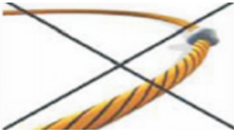
Glue-Fixed Installation (Prone to Cable Damage)
