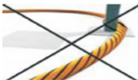
Metal-Tie Installations (Prone to Interference-Causing False Alarms)
